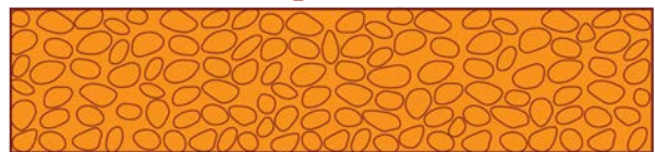
Open crystal structure at soldering temperature
